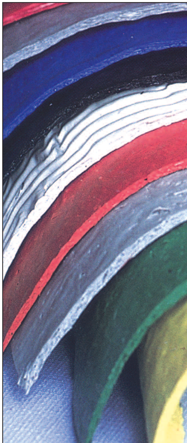
IDI SMC can be formulated with 10 – 60 percent glass content depending on the physical requirements of the application.
